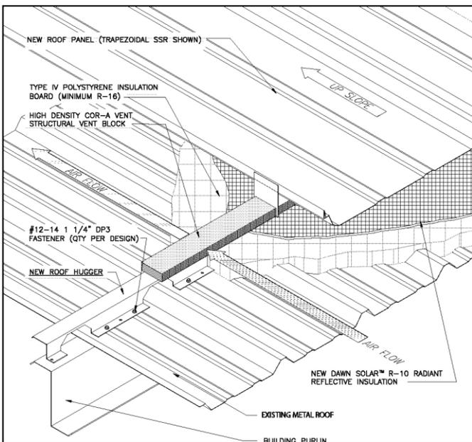
“SHR” installed over metal roof with Cor-A-Vent™ strip and rigid insulation between existing and new roofs
